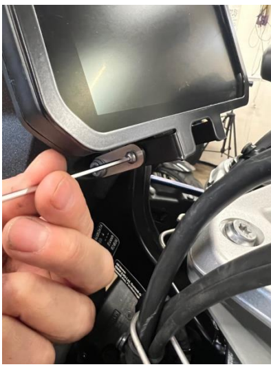
Step 5. Loosely insert the lower M4 fasteners on both sides.
