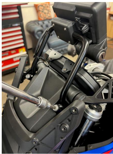
Step 6. Remove ONE prep for sat nav mounting fastener (you need the other to be still tight in place to hold your sat nav bar firm while you remove the fastener).
