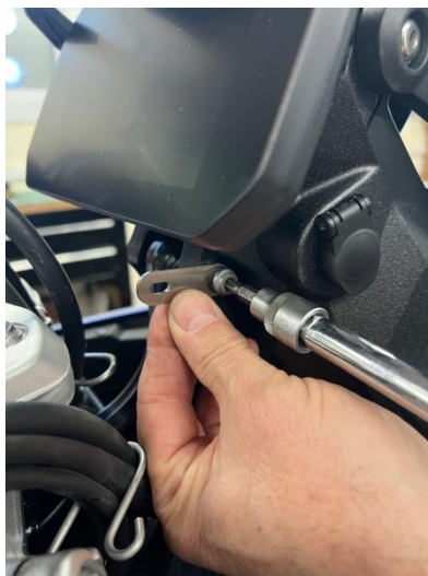
Step 3. Loosely Install the two supplied lower mounting extension brackets using the OE fasteners (note position of the slot is rearward).
